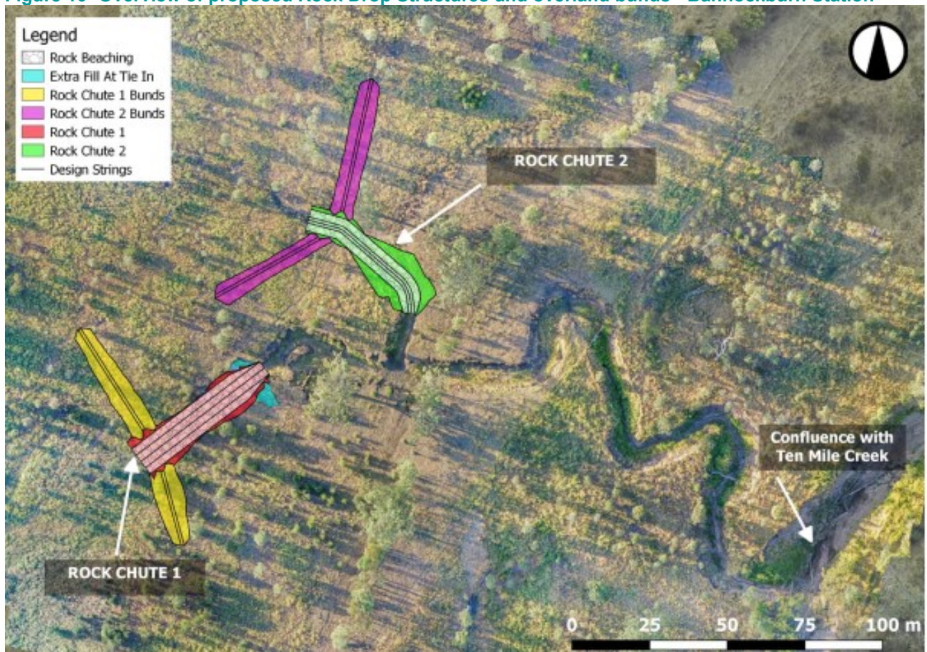
Figure 10- Overview of proposed Rock Drop Structures and overland bunds - Bannockburn Station
