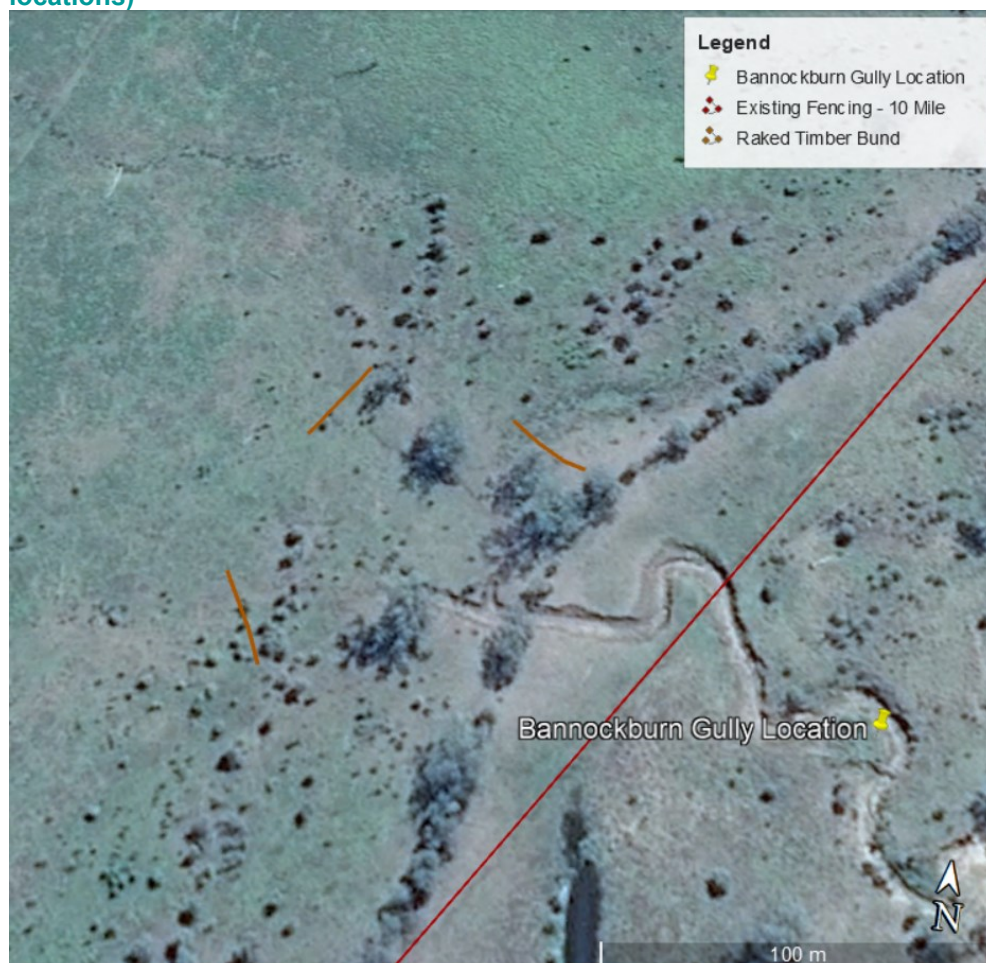
Figure 11- Overview of proposed timber raked check dam - Bannockburn Station (approximate locations)
