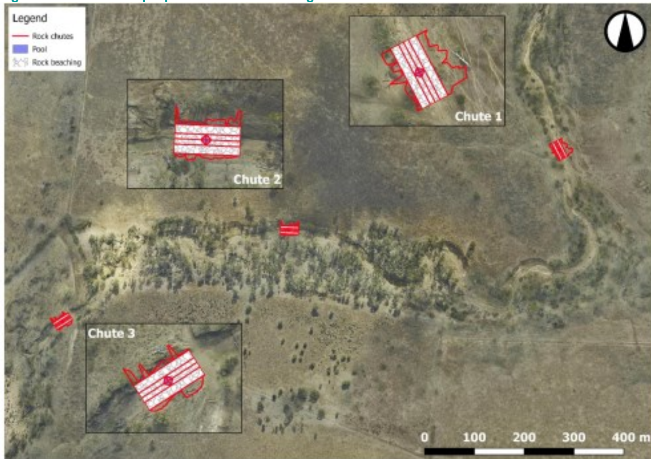
Figure 3 –Overview of proposed rock chute design- Mt. Fairview Station
