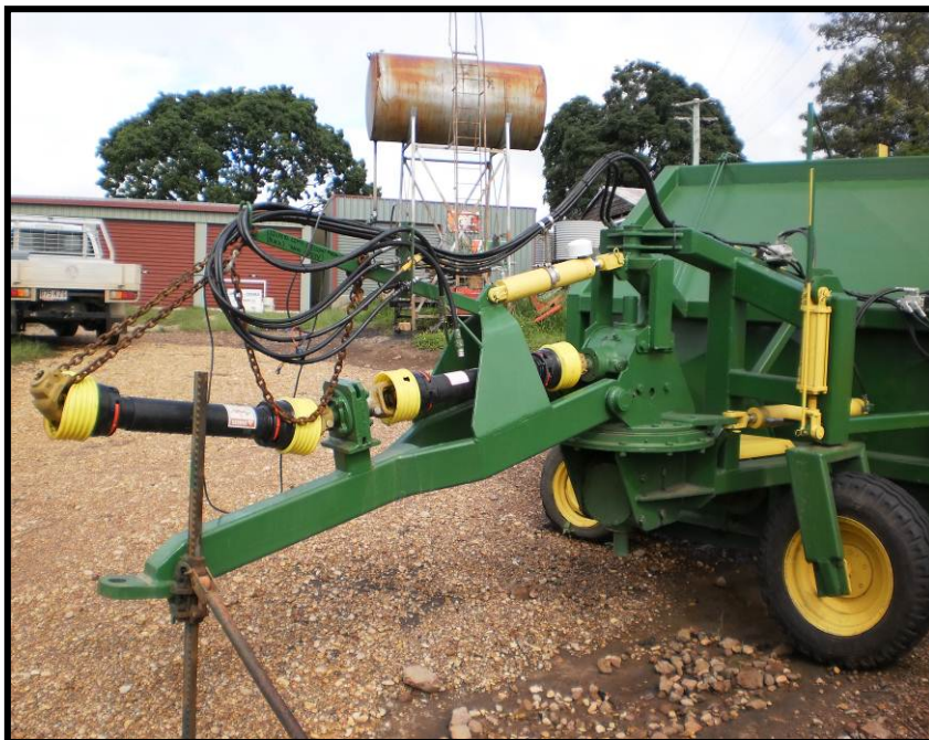
Figure 2. Novel end tow assembly, the ball race allows the tow bar to swing between end tow operation and mixing operation (90°). Conventional mixers cannot be towed at any speed because the mixer is folded up and is unstable during towing. Note also the castor wheel with hydraulic height control.
