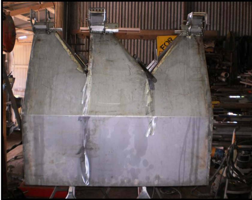
Figure 1. Photo of fertiliser boxes there are baffles inside to split the box into three sections, one large section for macronutrients and two small sections for micronutrients. The fertiliser is deposited on top of the rill during the mixing operation and mixed through.
