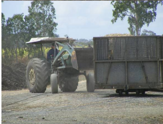
Photo 9: Home-made loader bucket on three-point linkage
