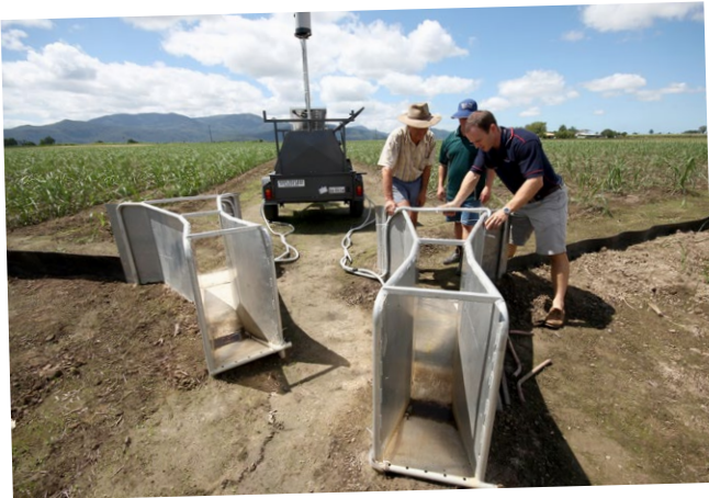
An automatic water sampling set up on a cane farm in the Herbert.
