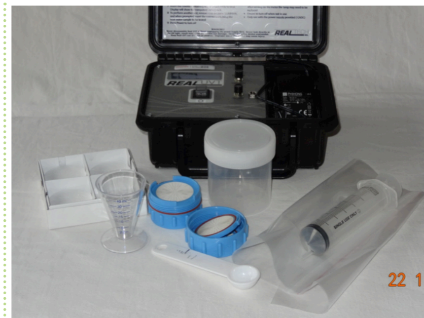
Figure 1: Components of the field UV method testing kit. From front left to right, 47 mm diameter, 45 µm glass fibre filter paper discs, 40 mL measuring cup, 47 mm filter disc holder, one teaspoon measure, one capped plastic container for shaking the solution, one 60 mL syringe for forcing the liquid through the filter, and a sealed plastic bag for pulverising the soil sample. Portable UV spectrophotometer is at the rear.
